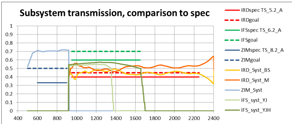
Figure 9. Transmission budget for the SPHERE science channels ZIMPOL (light blue) in the visible and IRDIS (orange and yellow for each of the two dual imaging channels) and the IFS (light and dark green for the YJ and YJH channels, respectively) in the infrared. The dark blue, red and light green lines indicate specified (full lines) and goal (broken lines) transmission levels for each of the channels.
